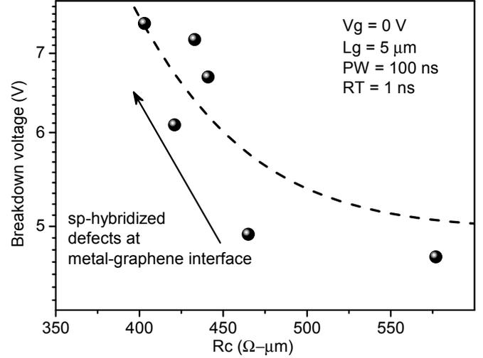
Fig. 9: Dependence of breakdown voltage on contact resistance. Devices demonstrate a down-scaling of breakdown voltage with increasing contact resistance. Engineering the contacts by creating *sp*-defects improves the metal-graphene bonding, which eventually reduces the resistive heating at contacts and increases the breakdown voltage.
