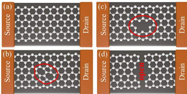
Fig. 6: A pictorial representation of defect-evolution in graphene. (a) pristine lattice of graphene; (b) topological defects (5-7) shown in red; (c) maximum scattering and oxidation happens at the defect site (5-7), resulting in increase in defect density; (d) further increase in time/field causes complete oxidation of the lattice. (c) and (d) constitute time-dependent defect-by-defect breakdown.
