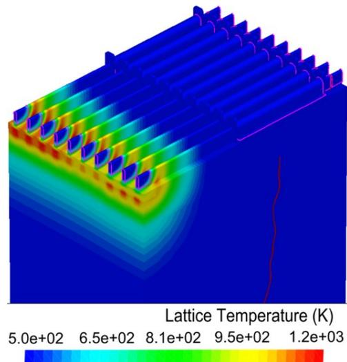
Figure 12: Lattice Temperature profile in a multi-fin (with number of fins = 10) DeFinFET device extracted at  $I_{TLP} = 4$  mA/ $\mu$ m at 100ns, depicting non-uniform current conduction under transient current stress. A fin to fin variation of the n+ drain doping is investigated.
