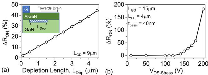
**Fig. 10.** (a) Impact of selectively depleting the 2-DEG, by emulating a localized charge sheet below 2-DEG, on the  $\Delta R_{ON}$  performance of the HEMT. For the simulation exercise, the depleted region had 3 orders of magnitude lower carrier density as compared to the 2-DEG channel carrier density. (b) Results of TCAD simulations of the device with conditions similar to experimental setup and considering dynamic trapping of electrons in acceptor-type GaN buffer traps.
