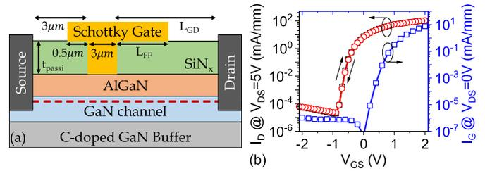
Fig. 1. (a) Schematic of the Schottky-gated AlGaIn/GaN HEMTs under test. (b) Absence of hysteresis in the dual sweep transfer ( $I_D - V_{GS}$ ) and gate leakage ( $I_G - V_{GS}$ ) characteristics depicts superior gate-stack quality of the HEMTs under test. Device dimensions: gate–drain distance ( $L_{GD}$ ) = 15  $\mu m$ , field plate length ( $L_{FP}$ ) = 4  $\mu m$ , passivation thickness ( $t_{passi}$ ) = 20 nm.
