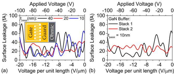
**Fig. 6.** Surface leakage measured using a specifically designed test structure (shown in inset), as reported by Tan *et al.* [22]. It shows negligible dependence on (a) passivation thickness ( $t_{\text{passi}}$ ) and (b) C-doping in GaN buffer. The distance between the gate and guard structure is  $5 \mu\text{m}$ .
