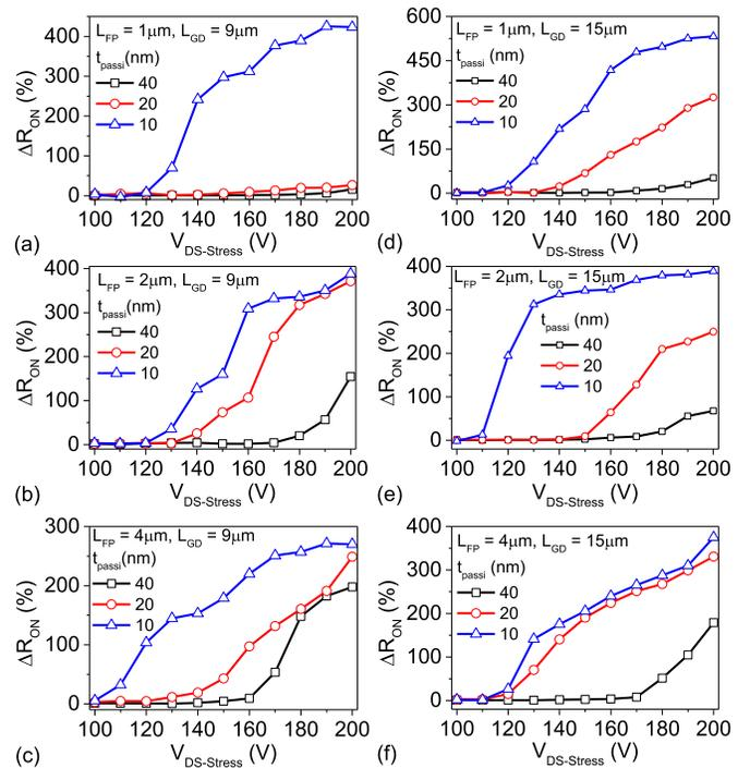
**Fig. 5.**  $\Delta R_{ON}$  extracted for devices as a function of passivation thickness ( $t_{passi}$ ) for  $L_{GD}$  ( $\mu\text{m}$ ),  $L_{FP}$  ( $\mu\text{m}$ ) values of (a) 9, 1, (b) 9, 2, (c) 9, 4, (d) 15, 1, (e) 15, 2, and (f) 15, 4. The dynamic  $R_{ON}$  and  $V_{cr}$  show a distinct dependence on  $t_{passi}$ , irrespective of  $L_{GD}$  and  $L_{FP}$ . The HEMTs were stressed for 100  $\mu\text{s}$ .
