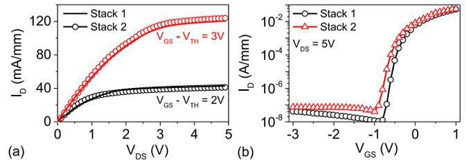
**Fig. 11.** Typical (a)  $I_D - V_{DS}$ , and (b)  $I_D - V_{GS}$  characteristics of the Schottky-gated HEMTs fabricated on stacks with different C-doping (Stack 1 and Stack 2). It shows similar output and transfer characteristics for devices on both the stacks.
