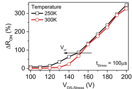
**Fig. 13.** Dynamic  $R_{ON}$  of the HEMTs extracted for different temperatures depicts a reduction in critical voltage for  $\Delta R_{ON}$  as temperature is reduced. Device parameters are  $L_{GD} = 15 \mu m$ ,  $L_{FP} = 1 \mu m$  &  $t_{passi} = 20 nm$ . Device was stressed for  $100 \mu s$ .
