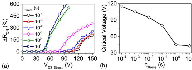
**Fig. 3.** (a) Dynamic  $R_{ON}$  of the HEMTs as a function of drain stress voltage for different OFF-state stress time. It shows a stress time-dependent critical voltage ( $V_{cr}$ ) beyond which  $\Delta R_{ON}$  increases significantly. (b) Reduction in  $V_{cr}$  with increase in stress time.  $V_{cr}$  is however seen to saturate for  $t_{Stress}$  beyond 1 s. The device parameters are  $L_{GD} = 15$   $\mu\text{m}$  and  $L_{FP} = 4$   $\mu\text{m}$ .
