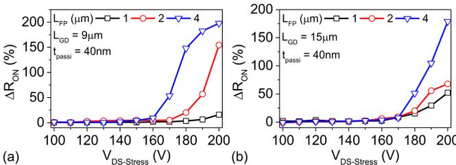
**Fig. 4.** Dynamic  $R_{ON}$  characteristics as a function of field plate length ( $L_{FP}$ ) for a gate-drain distance ( $L_{GD}$ ) of (a) 9  $\mu\text{m}$  and (b) 15  $\mu\text{m}$ . A dependence of  $V_{cr}$  on lateral device design parameters can be observed. These HEMTs had a 40 nm  $\text{SiN}_x$  passivation and were stressed for 100  $\mu\text{s}$ .
