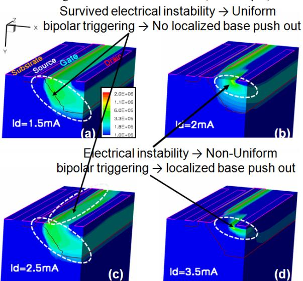
Figure 7: Electric field (V/cm) plot (Width=5 $\mu\text{m}$ ) at different TLP level. Figure shows uniform bipolar triggering after base push out in 2D plane for few pulses (Fig. 7a and 7c), whereas filament, shrink at the corner, (Fig. 7b and 7d) leads to higher carrier modulation (causes deep snapback) for other pulses.
