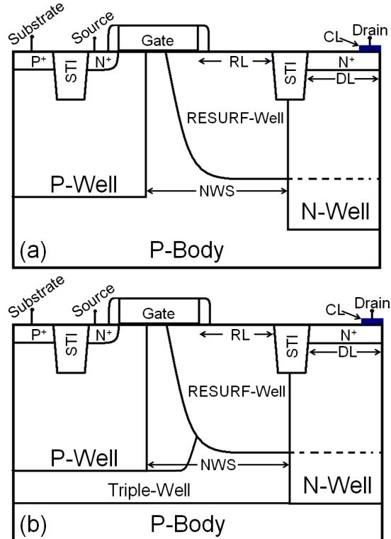
Fig. 13: Various modified RESURF DeMOS devices. (a) Device with extra STI and N-Well - "Type 2" (b) Further modified device with added triple well- "Type 3".
