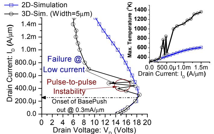
Fig. 2: Simulated (2D and 3D) TLP characteristics of RESURF DeNMOS under HBM like ESD condition. Width in 3D simulation is chosen to 5  $\mu\text{m}$ . 3D simulations are done with single contact strip.
