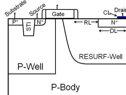
Fig. 1: RESURF DeNMOS device structure (*Type I*).
