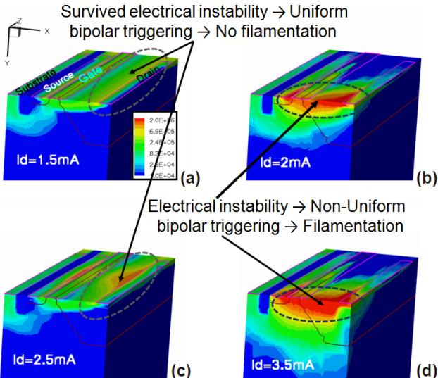
Fig. 4: Current density plot (A/cm<sup>2</sup>). Figure describes two different conditions- (i) uniform bipolar triggering along the width and (ii) non uniform triggering or current filamentation (Width=5 $\mu\text{m}$ ).
