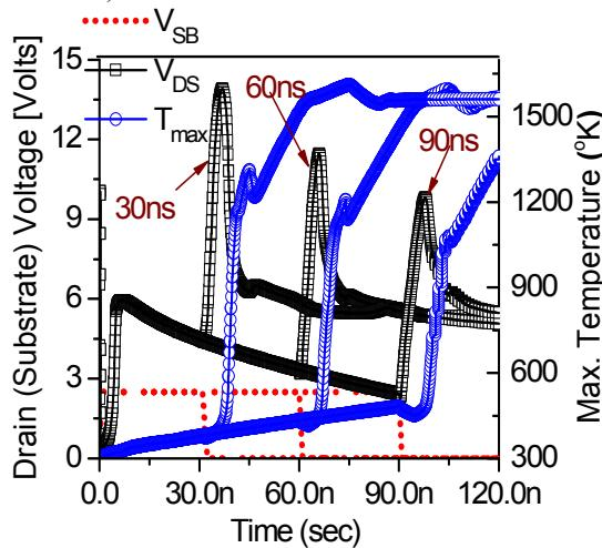
Figure 11: Validation of filament behavior and failure model.
