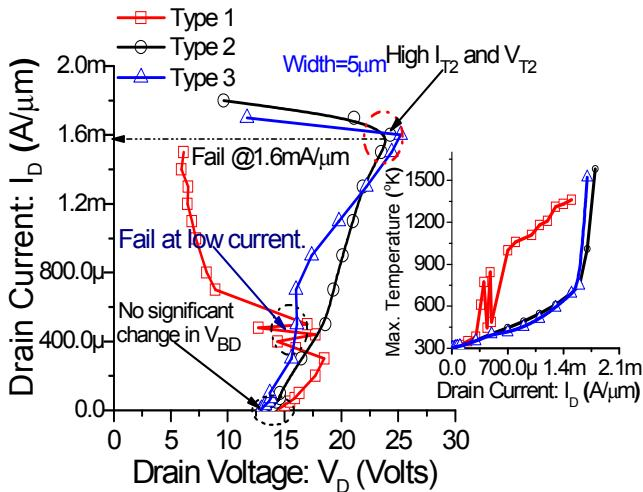
Fig. 14: Comparison of simulated TLP characteristics of standard and modified RESURF devices. Modified RESURF device show higher  $I_{T2}$  and ESD window.
