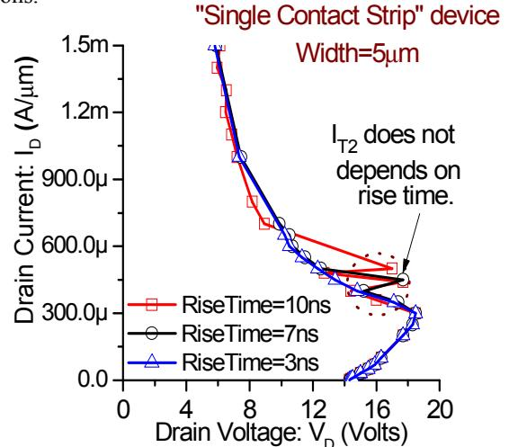
Figure 5: Dependence of simulated TLP characteristics on rise time (or pulse shape). Pulse-to-pulse instability depends on rise time of pulse, eventually on pulse shape.
