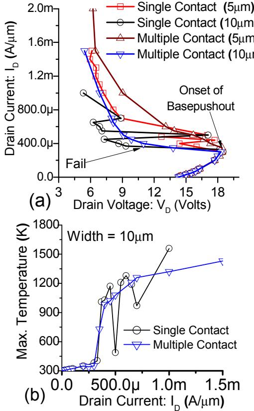
Fig 3: (a) Simulated TLP characteristics (HBM) of single contact strip and multiple contact strip devices with different widths. Devices with higher width fail at the onset of base push out driven snapback. (b) Shows Temperature rise with increasing TLP current for device with width = 10 $\mu\text{m}$ .
