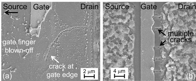
Fig. 12. (a) Post failure SEM image of device failed under OFF-state in UV exposure. Figure shows cracking underneath gate blew-off the gate finger which was already under compressive stress as clear from Raman plots. (b) SEM image of device failed in OFF-state under dark. Multiple damages observed in gate-drain region reveal failure due to non-uniform trapping and stress distribution along device width as shown in Fig. 6(a)–(c).
