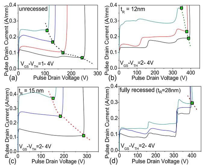
Fig. 9. (a) SOA boundary of devices with different gate recess depth ( $t_R$ ). (a) Figures shows narrow SOA boundary in HEMT without recess. (b)-(d) shows SOA of devices with increasing recess depth. Figure reveals that with gate recess the SOA broadens however, with fully recessed gate as in (d) device failure occurred at a fixed drain voltage irrespective of the gate bias and reveals field limited SOA in fully recessed structure.
