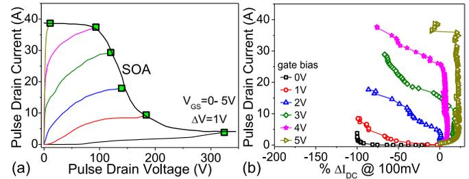
Fig. 2. (a) Pulse IV characteristics of a commercial GaN HEMT with SOA boundary marked. (b) Percentage change in linear drain-to-source DC current ( $I_{DC}$ ) measured at 100 mV  $V_{DS}$  under 2 V  $V_{GS}$ , after each stress pulse is applied at drain. Severe degradation is observed at different gate bias with highest degradation ( $\sim 100\%$ ) under OFF-state.
