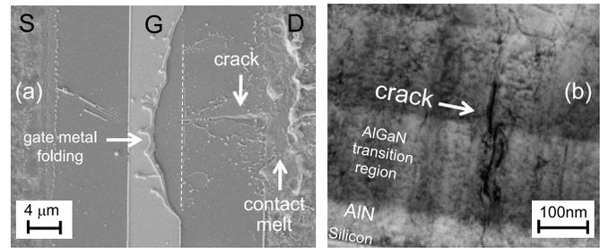
Fig. 15. (a) OFF-state failure occurred with crack in gate-drain region with gate metal folding. (b) TEM cross-section image taken across the crack along the white dotted line in (a), shows damage in bulk reaching till Si substrate.
