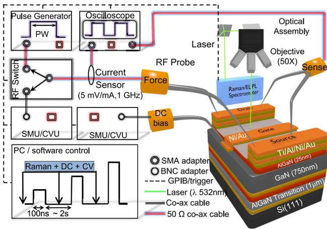
Fig. 1. Experimental set-up with integrated Raman and sub- $\mu$ s pulse generator used for pulse IV characterization to determine SOA behavior of AlGaIn/GaN HEMTs. Schematic of HEMT shows details of different layers present in the AlGaIn/GaN stack. The stack is capped with a 3 nm GaN cap (not shown).
