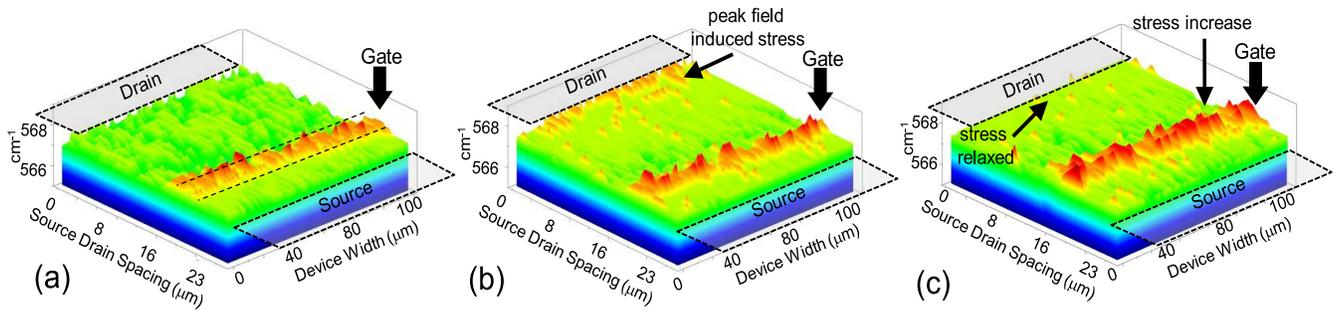
Fig. 6. (a) Raman map captured in source-drain region of pristine device, before stress. On the fly Raman map was captured during OFF-state stress ( $V_{DS}$  60V @  $V_{GS}$  -6V) (b) in dark and (c) with UV illumination on device.
