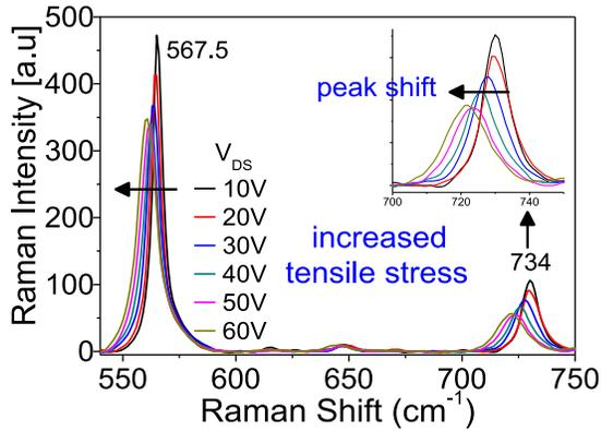
Fig. 7. Raman spectra spot measured, under ON-state, at gate edge towards drain at different drain stress. Left shifting in  $E_{2-H}$  ( $567.5 \text{ cm}^{-1}$ ) and  $A_{1-LO}$  ( $734 \text{ cm}^{-1}$ ) Raman peaks of GaN reveal increased tensile stress at gate edge with increase in drain voltage.
