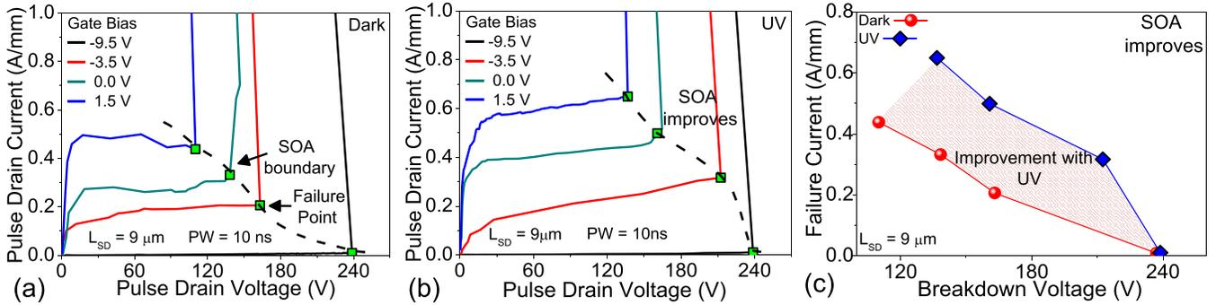
Fig. 1. Pulse  $I$ - $V$  characteristics of HEMT (a) under dark condition and (b) with UV exposure. Failure point shown here marks the SOA boundary. (c) Variation in SOA boundary of HEMT stressed under dark and UV condition. As evident, SOA boundary of device widens under UV light.
