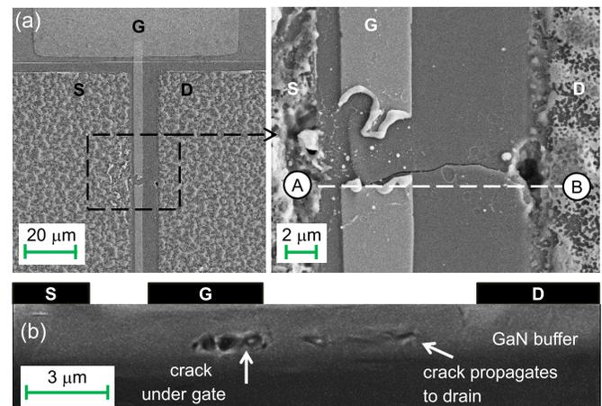
**Fig. 15.** (a) SEM image of HEMT failed under UV condition, stressed using 10-ns wide pulses depicting damage in G-D region. (b) Cross-sectional SEM image taken along line “A-B” depicts cracks underneath the drain side of gate edge which propagated toward the drain.
