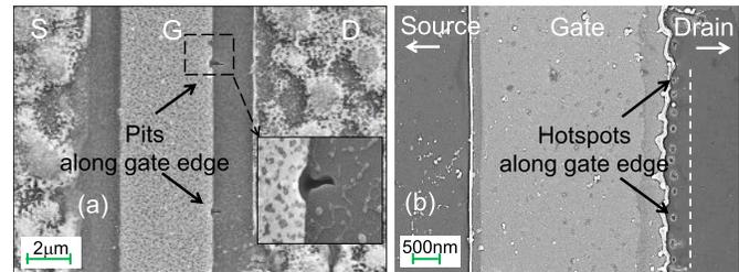
**Fig. 14.** (a) SEM image of HEMT which failed at 100 ns under UV light in OFF-state condition. Pits get formed at multiple locations along the gate edge toward drain. (b) SEM image of HEMT with  $7 \mu\text{m}$   $L_{SD}$  which failed at 100 ns under UV condition in ON-state. Images reveals continuously distributed hotspots along the gate edge toward drain. Gate metal folds up at hotspot locations. No damage is observed at source side.
