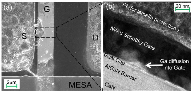
**Fig. 13.** (a) SEM image of HEMT with  $11 \mu\text{m}$   $L_{SD}$ , which failed under dark condition when stressed with 10-ns-wide pulses under ON-state. (b) Cross-sectional TEM taken in the dotted area of the damaged S-G region reveals Gallium out diffusion from GaN cap into Ni/Au Schottky gate.
