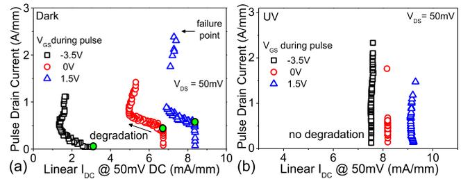
**Fig. 3.** (a) Linear drain-to-source current measured after each stress pulse of 100-ns duration applied at drain of a device of  $L_{SD}$  7 μm under (a) dark and (b) UV condition. Unique current degradation trend can be observed under dark condition at different gate biases, which is absent under UV illumination.
