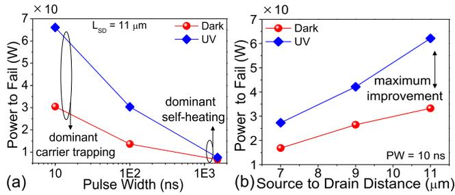
**Fig. 2.** (a) Power to fail as a function of PW extracted under dark and UV condition. While exhibiting power law behavior presence of UV improves power to fail at shorter pulses. (b) Power to fail as a function of source–drain spacing. It increases linearly with  $L_{SD}$  and shifts upward with UV exposure.
