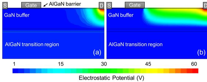
Fig. 7. Electrostatic potential distribution in gate–drain region simulated for (a) high buffer trap density ( $10^{18} \text{ cm}^{-3}$ ) and (b) low buffer trap density ( $10^{15} \text{ cm}^{-3}$ ) in GaN buffer, extracted at  $V_{DS} = 60 \text{ V}$  and  $V_{GS} = -6 \text{ V}$ .
