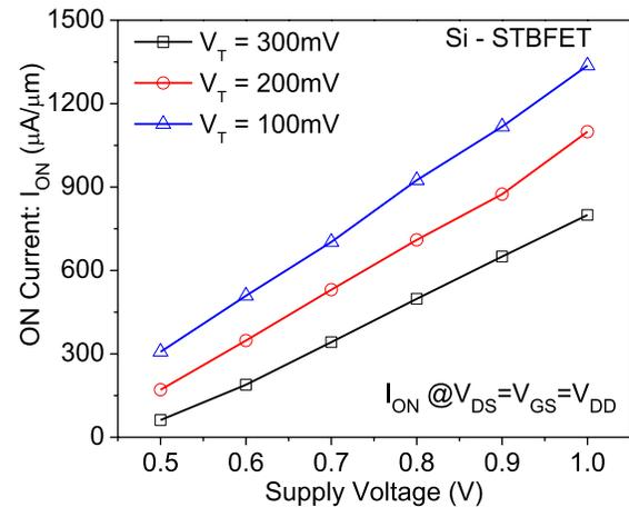
Fig. 3. Silicon STBFET (N-Type) ON current as a function of supply voltage for different threshold voltages. When supply voltage varies from 1 to 0.5 V, the ON current decreases by five times for a  $V_T = 100\text{-mV}$  device. Sandwich barrier tunnel FET using a SiGe source is an implementation of an area scaled TFET.
