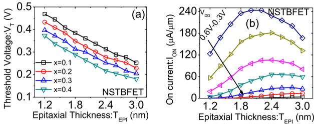
Fig. 7. Impact of epitaxial thickness on (a)  $V_T$  with different values of Ge for a constant 0.5 V supply and (b)  $I_{ON}$  with different value of supply voltage (varied from 0.6 to 0.3 V in 0.05 V step) for a fixed 30% Ge content ( $x$ ).
