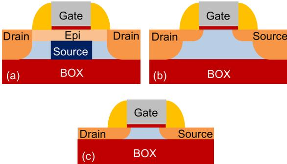
Fig. 4. Schematic representation of cross section of the devices used in this paper with  $L_G = 20$  nm. (a) STBFET. (b) High performance MOSFET (MOS-HP). (c) Low power MOSFET (MOS-LP). In STBFET devices, source is n++ (p++) in the case of N-type (P-type) operation.
