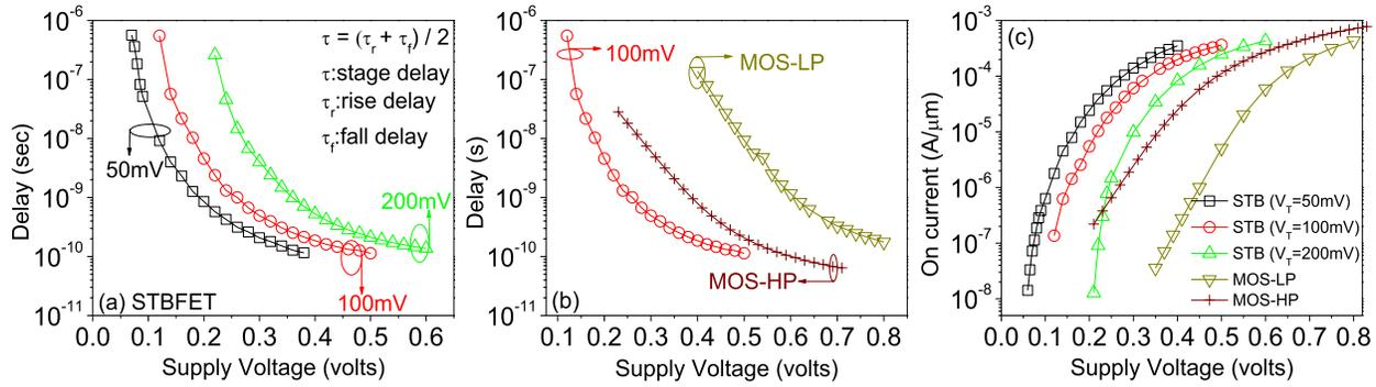
Fig. 11. Delay versus supply voltage for (a) STBFET devices, (b) for MOSFETs and TFET, and (c)  $I_{ON}$  at  $V_{GS} = V_{DS} = V_{DD}$ . Roughly delay is given by  $C_L V_{DD} / I_{ON}$  hence for a fixed  $C_L$  (2.4 fF) device that shown in better  $I_{ON}$  for a given  $V_{DD}$  gives a better performance.
