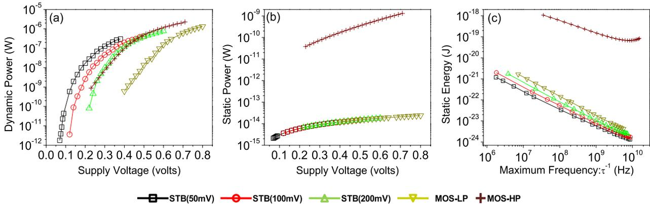
Fig. 12. (a) Dynamic power, (b) static power, and (c) static energy ( $E_{st} = P_{st} \times \tau$ ) where  $\tau$  being the stage delay. A MOS-HP dissipates more energy in idle state than the rest of the devices. This becomes worse at low operating frequencies making these devices unsuitable for applications where high battery life is required in idle state.
