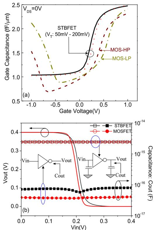
Fig. 10. (a) Simulated gate capacitance of the devices. (b) Inverter transfer characteristics and capacitance of a STBFET and a MOSFET. As maximum gate capacitance value lies 2–2.5 fF/ $\mu\text{m}$  for all the devices having  $W_p/W_n = 3$  with  $W_n = 30$  nm, absolute device capacitance ( $\sim 10^{-17}$  F) is always of two orders lower compared with the load capacitance  $C_{INT}$  (2.4 fF).
