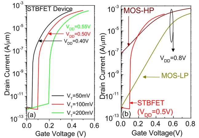
Fig. 9. Simulated transfer characteristics (a) for area scaled device with varying  $V_T$ , where  $V_T$  is defined at a gate voltage where the device exhibits a sharp rise in drain current (arrows point drain voltage used). (b) Both MOSFETs and an area scaled device ( $V_T = 100$  mV).
